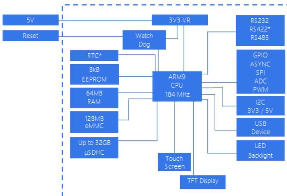
Figure 1 - Circuit Block Diagram.
