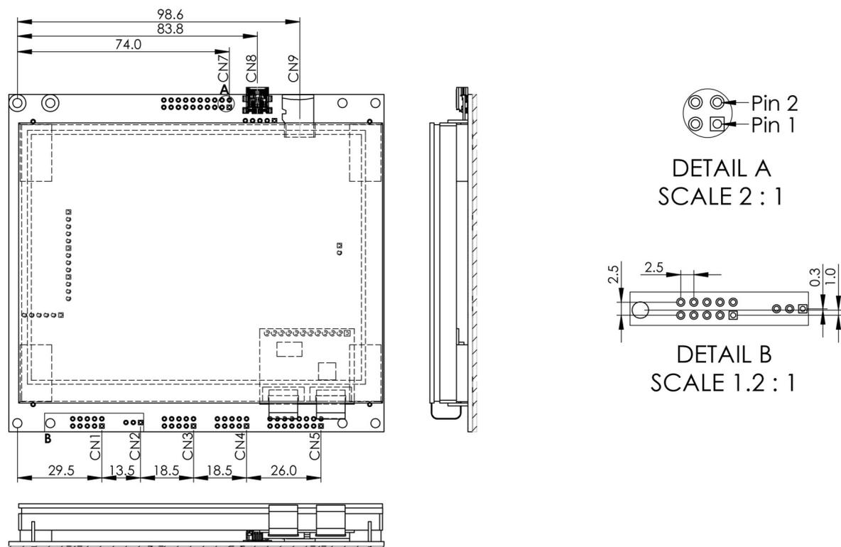
Figure 5 - TU640x480C-K61XA1XX Connector Location drawing. Reference dimensions only.
