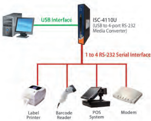
Connections of USB to Serial Media Converter
