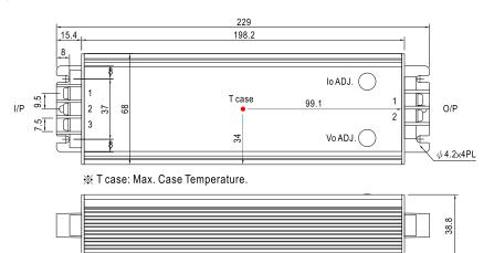
※ Output voltage and constant current level can be adjusted through internal potentiometer. (Can access by removing the rubber stopper on the case.)
