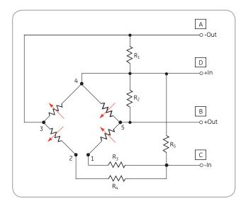
NPI-19 Series Constant Current schematic diagram
