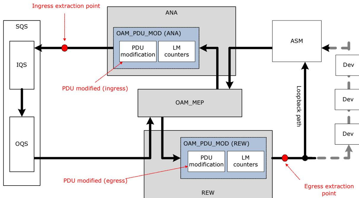
OAM PDUs extracted to the CPU at the ingress extraction point reflect the changes made to the PDU by the OAM\_PDU\_MOD (ANA). Likewise OAM PDUs extracted to the CPU at the egress extraction point reflect the changes made to the PDU by the OAM\_PDU\_MOD (rewriter).
