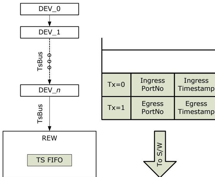
The bus passes through all port modules and terminates in a timestamp FIFO in the rewriter. If the analyzer has decided to do a two-step operation, the rewriter pushes two entries into the FIFO. The first entry contains the egress time stamp and the egress port number; the second entry contains the ingress time stamp and the ingress port number. In addition, a flag indicates whether the entry contains ingress or egress information.
