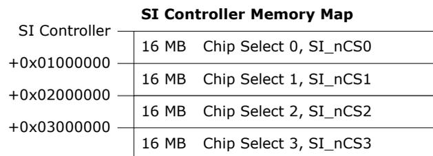
The SI boot controller can be reconfigured for 32-bit address mode through SPI\_MST\_CFG.A32B\_ENA. In 32-bit mode, the entire SI region of 256 megabytes (MB) is addressed using chip select 0.
