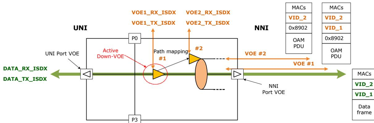
A bidirectional data flow (indicated using green) is mapped to a service Down-VOE (Down-VOE #1). The service is carried across a server layer monitored by Down-VOE #2. Two OAM PDU flows are illustrated:
