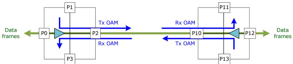
It shows the bidirectional OAM PDU flow between two Up-MEPs (shown using blue) and the bidirectional data frame flow being monitored by the two Up-MEPs (shown using green). The Up-MEP injects the Tx OAM in the ingress frame flow after the front port towards the queue system. This defines the point of the Up-VOE Tx lookup. Likewise Rx OAM frames are extracted from the egress frame flow directly from the queue system before reaching the front port. This defines the point of the Up-VOE Rx lookup.
