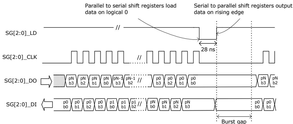
The SGPIO values are output in bursts followed by assertion of the SG[2:0]\_LD signal. Values can be output as a single burst or as continuous bursts separated by a configurable burst gap. The maximum length of a burst is  $32 \times 4$  data cycles. The burst gap is configurable in steps of approximately 1 ms, from 0 ms to 33 ms through SIO\_CFG.SIO\_BURST\_GAP\_DIS and SIO\_CFG.SIO\_BURST\_GAP.
