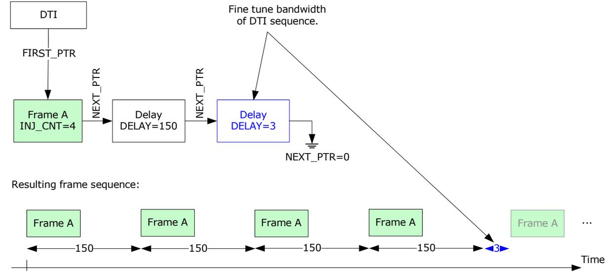
By combining the setting of  $INJ\_CNT$  and the  $DELAY$  value of the last delay depicted, the bandwidth of the DTI sequence can be controlled with high granularity, because the additional (blue) delay will only be applied for every  $INJ\_CNT$  injections of frame A.
