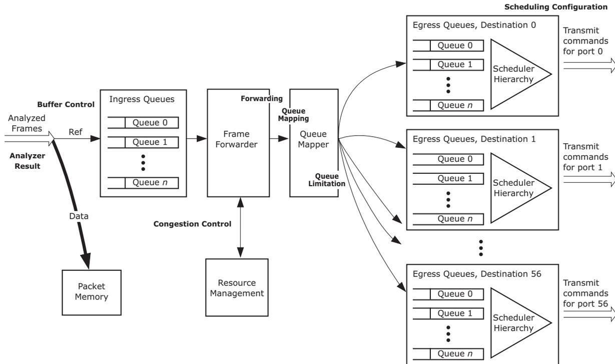
Frames are stored in the packet memory and linked into the ingress queue for the logical source port along with the analyzer result.
