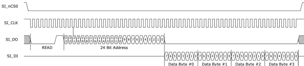
**FIGURE 3-18: SI READ TIMING IN FAST MODE**
