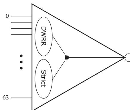
The lower indexes are arbitrated in the effort to achieve a bandwidth ratio between them. In this regard, the bandwidth can be measured in frames, data bits, or line bits (including IFG). Each input is configured with a cost setting, and the algorithm strives to give  $n$  times more bandwidth to input A than B, if the cost configuration for A is  $n$  times lower than B.
