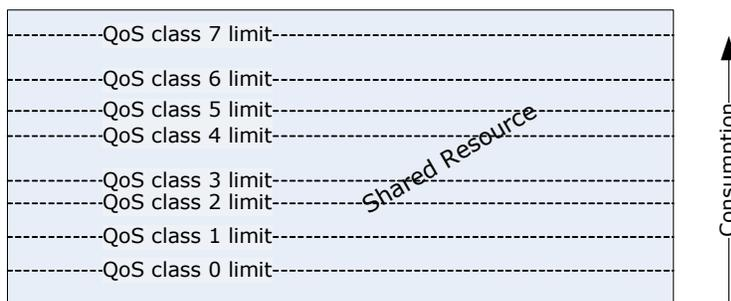
One important property of this mode is that higher QoS classes can block lower QoS classes. A congested flow with a high QoS class uses all of the shared resources up to its threshold setting and frame with lower QoS classes are thus affected (lower burst capacity).
