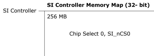
Reading from the memory region for a specific SI chip select generates an SI read on that chip select. The VCore-III CPU can execute code directly from Flash by executing from the SI boot controller's memory region. For 32-bit capable SI Flash devices, the VCore-III must start up in 24-bit mode. During the boot process, it must manually reconfigure the Flash device (and SI boot controller) into 32-bit mode and then continue booting.
