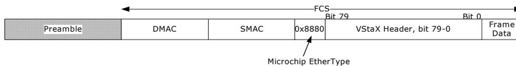
The layout of the 10-byte VStaX header is shown in the following illustration. In VStaX context, each switch in a stack is termed a unit.
