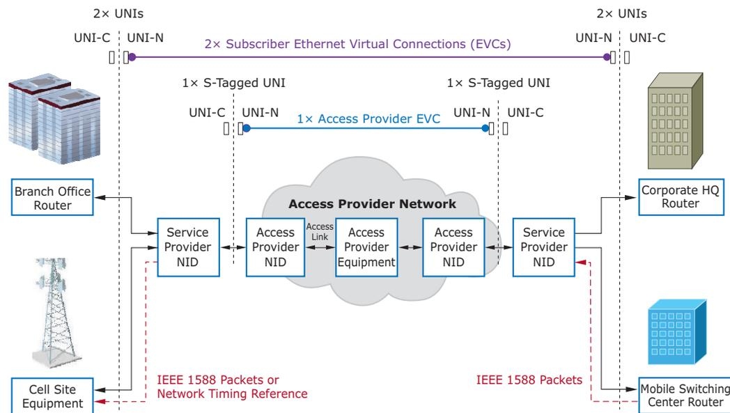
The following illustration depicts MEF-compliant E-access service. In this reference diagram, the access provider NID tunnels each remote UNI to the service provider network using UNI Tunnel Access Operator Virtual Connections (UTA OVCs).
