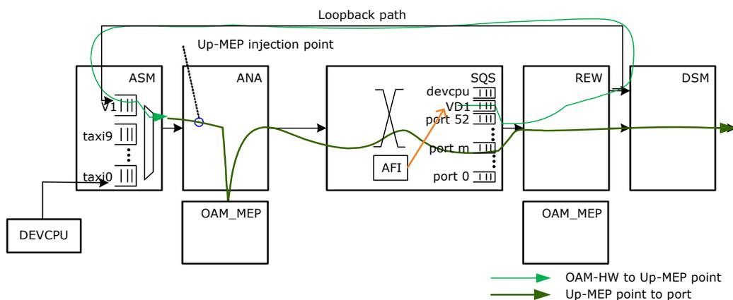
An Up-MEP injected frame must be masqueraded to appear as being received at the right ingress port (by setting IFH.MISC.PIPELINE\_ACT = INJ\_MASQ and IFH.FWD.SRC\_PORT = <masqueraded port>).
