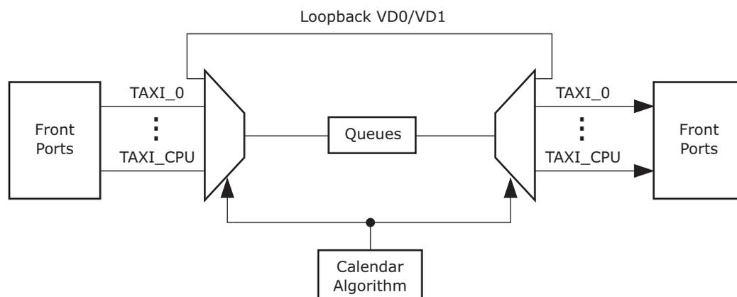
The front ports are connected to taxi busses and must be guaranteed bandwidth corresponding to their line speed. The internal CPU ports and loopback paths can operate up to 10 Gbps (7.5 Gbps for VD0).
