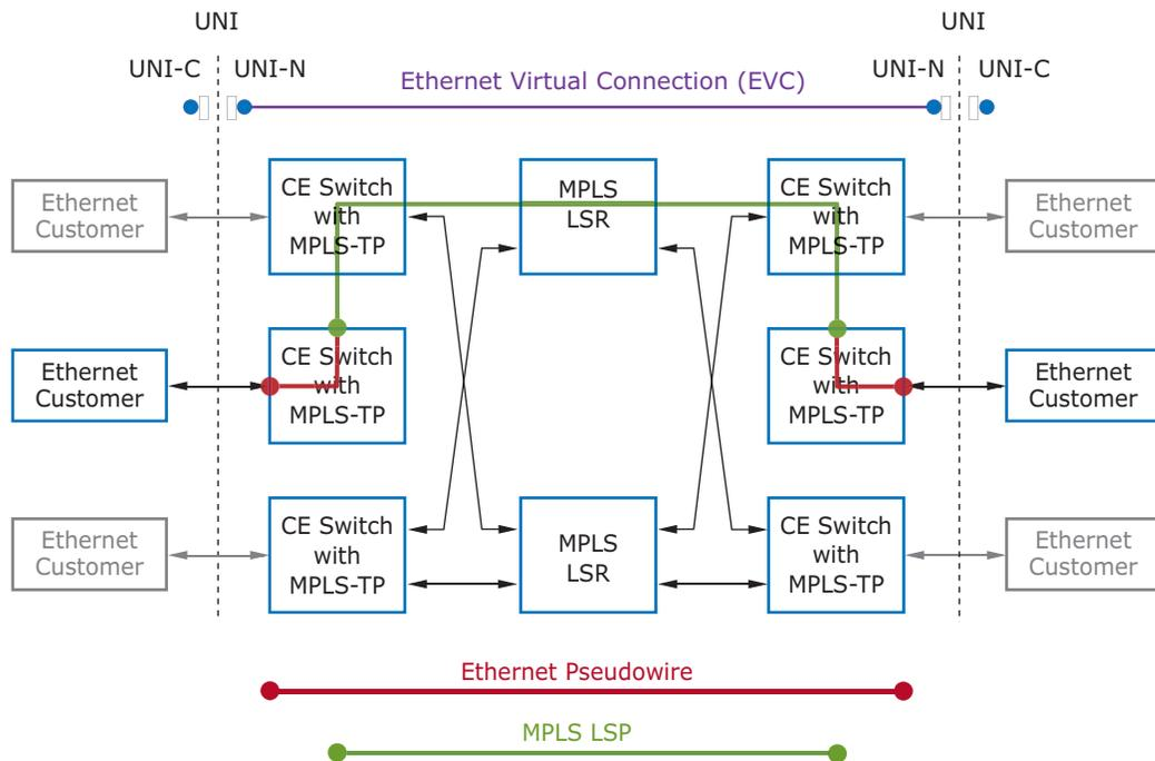
The Carrier Ethernet Switches initiating and terminating the pseudowire implement Provider Edge (PE) functions, providing Ethernet-to-MPLS and MPLS-to-Ethernet operations. These are also known as Pseudowire Label Edge Router (LER) operations. The PE switches also initiate and terminate the MPLS Label Switched Path (LSP) connection.
