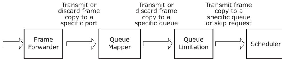
The queue limitation function checks the queue size against various configurable and dynamic values and may change a transmit request to a discard by canceling the request to the scheduler.
