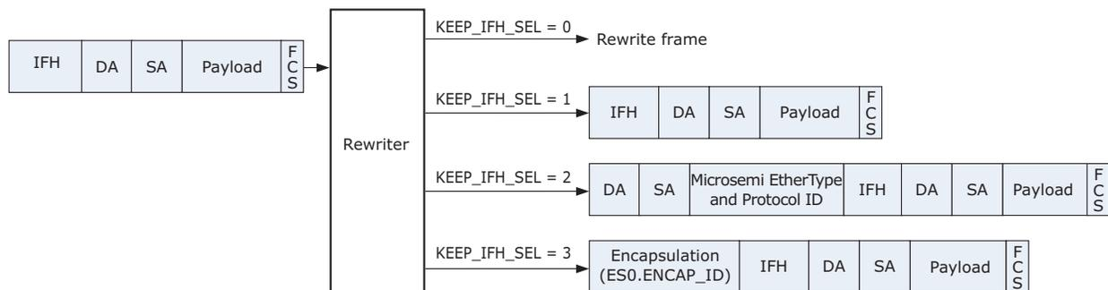
Frames are always formatted using KEEP\_IFH\_SEL = 1 when extracting frames to the internal CPU ports. This cannot be changed.
