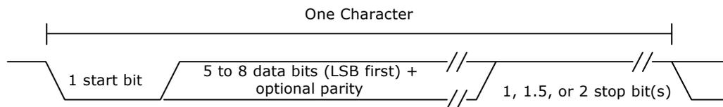
The number of data bits, parity, parity-polarity, and stop-bit lengths are all programmable using LCR.
