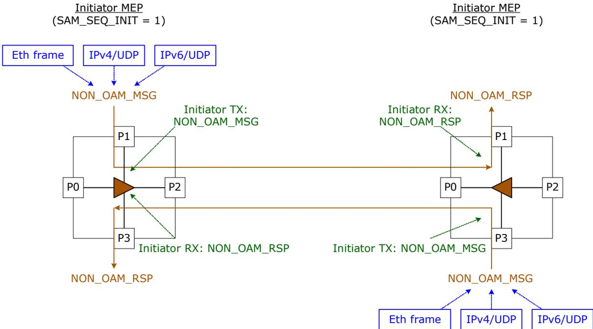
The SAM\_SEQ initiator transmits NON\_OAM\_MSG with sequence number PDUs towards the peer MEP (also configured as SAM\_SEQ Initiator). The peer MEP checks the sequence number of the Rx NON\_OAM\_RSPs and optionally extracts to the CPU.
