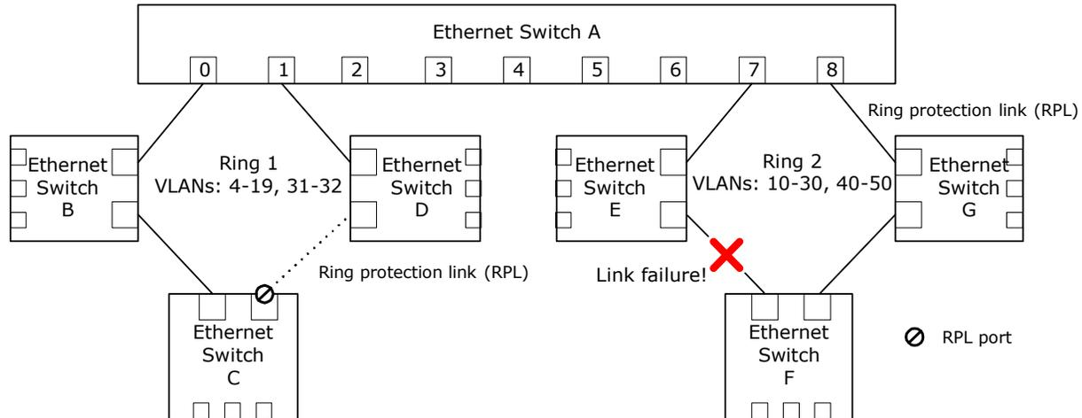
To avoid having to perform write access to the VLAN\_PORT\_MASKs of each of VID 10-30 and 40-50, VLAN TUPE can be used instead. The following table lists the VLAN TUPE parameters to reconfigure the VLAN table.
