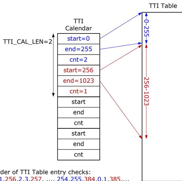
In the example, it takes  $(256/2) \times (1 + 2) \times 4 = 1536$  clock cycles to service all TTIs in the blue section. With a clock cycle of 4 ns, the TTIs in the blue section must not use ticks faster than  $1536 \times 4 = 6144$  ns.
