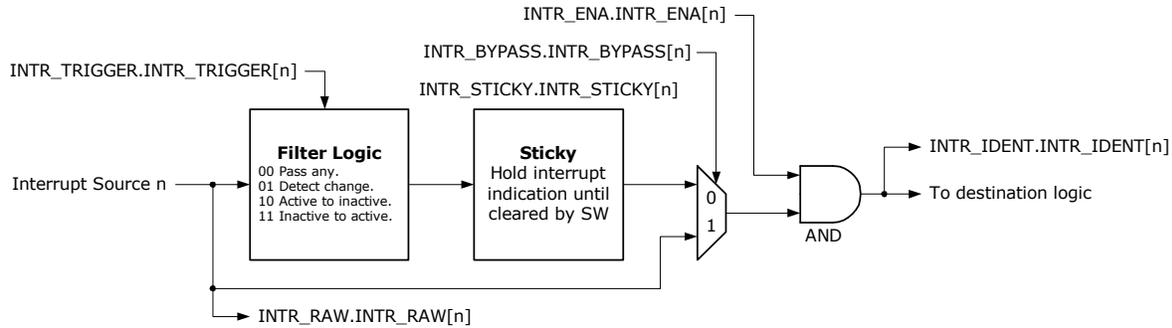
The current value of an interrupt source is available in `INTR_RAW.INTR_RAW[ $n$ ]`. `INTR_STICKY.INTR_STICKY[ $n$ ]` is set when the interrupt controller detects an interrupt. There are two detection methods:
