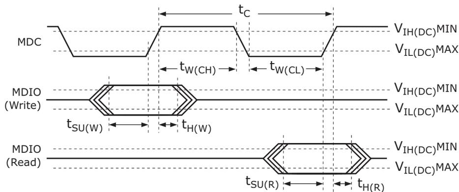
The set up time of MDIO relative to the rising edge of MDC is defined as the length of time between when the MDIO exits and remains out of the switching region and when MDC enters the switching region. The hold time of MDIO relative to the rising edge of MDC is defined as the length of time between when MDC exits the switching region and when MDIO enters the switching region.
