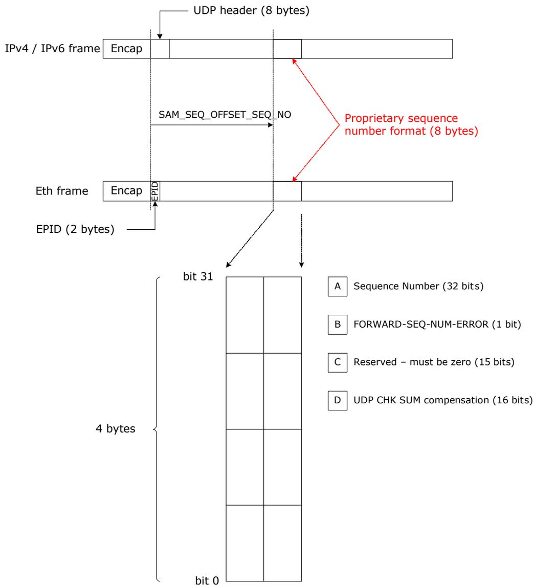
The location of the sequence number in the SAM\_SEQ frames is configured as a 16-bit offset from the beginning of the SAM\_SEQ PDU. Depending on the frame type the first byte of the SAM\_SEQ PDU is defined as:
