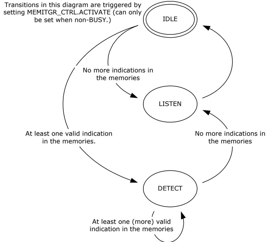
The first time after reset that MEMITGR\_CTRL.ACTIVATE is set, the monitor resets the detection logic in all the memories and transitions directly from IDLE to LISTEN state.
