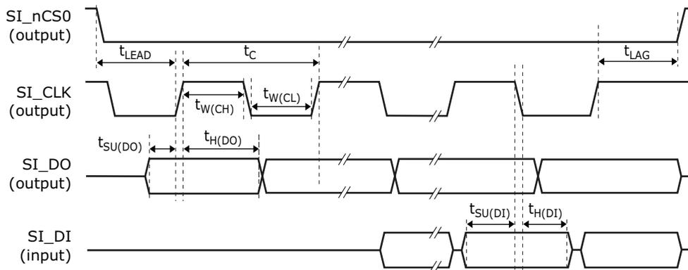
All SI signals comply with the specifications shown in the following table. The SI input timing requirements are requested at the pins of the devices.
