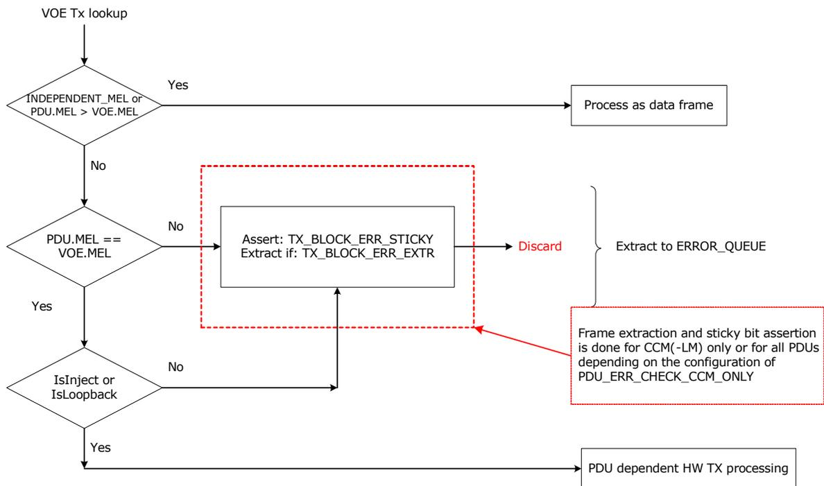
OAM PDUs discarded by the Tx validation are counted in VOP:VOE\_STAT:TX\_OAM\_DISCARD.TX\_FRM\_DISCARD\_CNT. At the same time, the VOP:VOE\_STAT:OAM\_TX\_STICKY.TX\_BLOCK\_ERR\_STICKY bit is asserted, and the frames can optionally (VOP:VOE\_SYAY:PDU\_EXTRACT.TX\_BLOCK\_ERR\_EXTR) be extracted to the CPU\_ERR\_QU.
