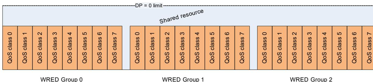
The following illustration shows an example of the WRED profiles for a QoS class within a WRED group. Thresholds are shown for DP = 2 only.
