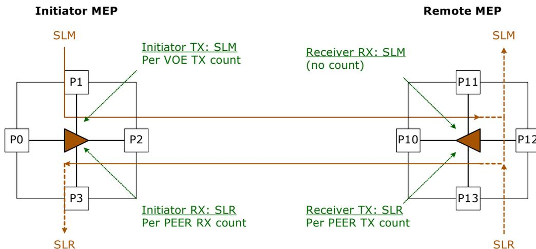
SLR PDUs transmitted from the Remote MEP can be either SLM PDUs looped by the VOE or SLR PDUs injected by the CPU. The Initiator MEP counts the number of Tx SLM PDUs. There is a dedicated counter for this purpose. The Remote MEP loops the SLM to SLR PDU, but no counters are implemented to count the incoming Rx SLM frames. The standard assumes that the Rx SLM count is identical to the Tx SLR count mentioned in the following:
