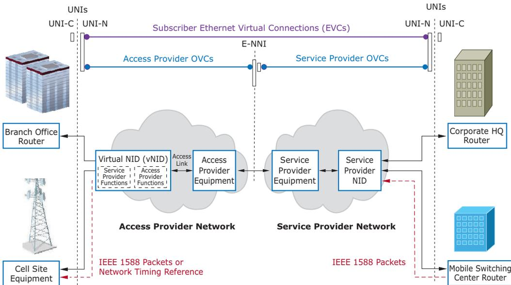
Microsemi's Carrier Ethernet switch family is optimized for delivery of MEF EVCs that are based on the Virtualized Service Aware Architecture (ViSAA™). MEF-compliant features include dual-rate policing, dual-rate shaping, statistics, and hardware-based OAM. Hierarchical QoS supports these features at the EVC and UNI/E-NNI level. In addition, Microsemi's Carrier Ethernet switches support the virtual NID model.
