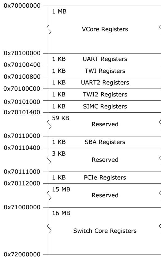
The registers in the 0x70000000 through 0x70FFFFFF region are physically located inside the VCore-III system, so read and write access to these registers is fast (done in a few clock cycles). All registers in this region are considered fast registers.
