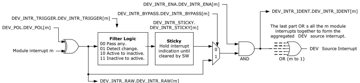
The module interrupt polarity is configurable in DEV\_INTR\_POL.DEV\_INTR\_POL[m].
