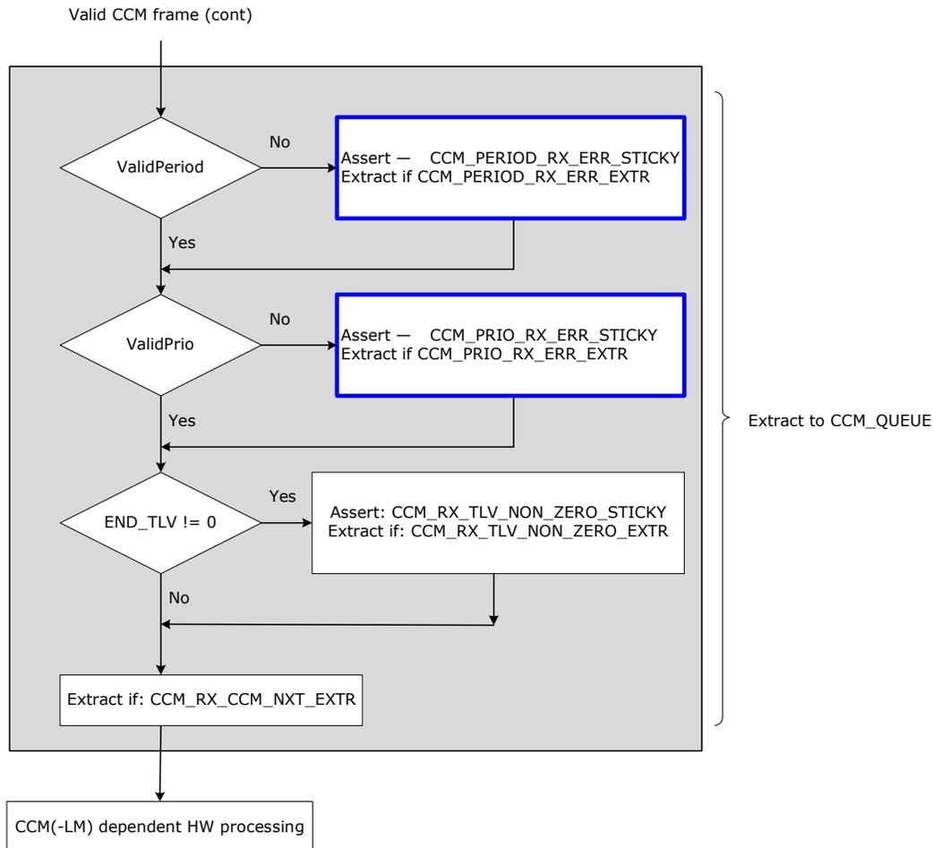
PDU's that are discarded due to failing the Rx validation are counted in VOP:VOE\_STAT:RX\_OAM\_DISCARD.RX\_FRM\_DISCARD\_CNT.
