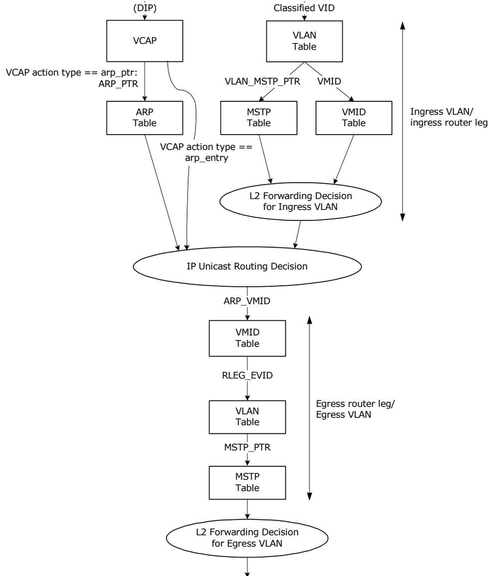
The following illustration provides an overview of the table lookups involved in IP multicast routing within the L3 part of the analyzer.
