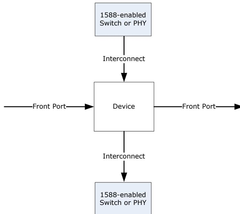
Hardware time stamping can update PTP frames coming from a standard front port without any 1588 support or from a partner device that does parts of the timing update. Each port is configured according to the partner device attached.
