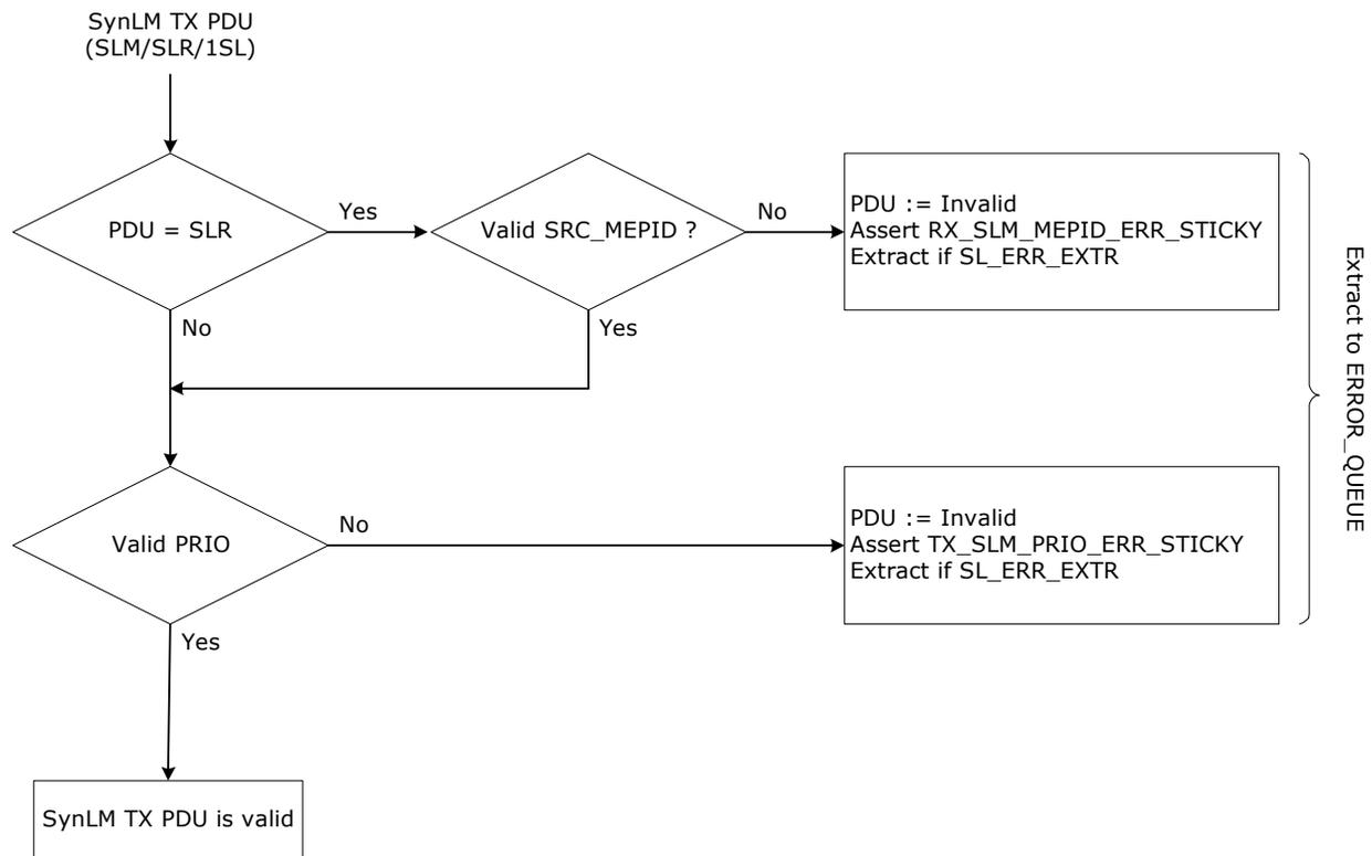
If the Tx PDU is SLR, the VOE validates the SLR.SRC\_MEPID:
