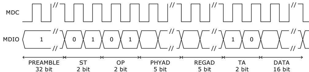
A read transaction is done in a similar way. First, read the DATA\_REG0 and then read the DATA\_REG1. As with a write operation. The switch core register read is not initiated before the DATA\_REG1 register is read. In other words, the returned read value is from the previous read transaction.
