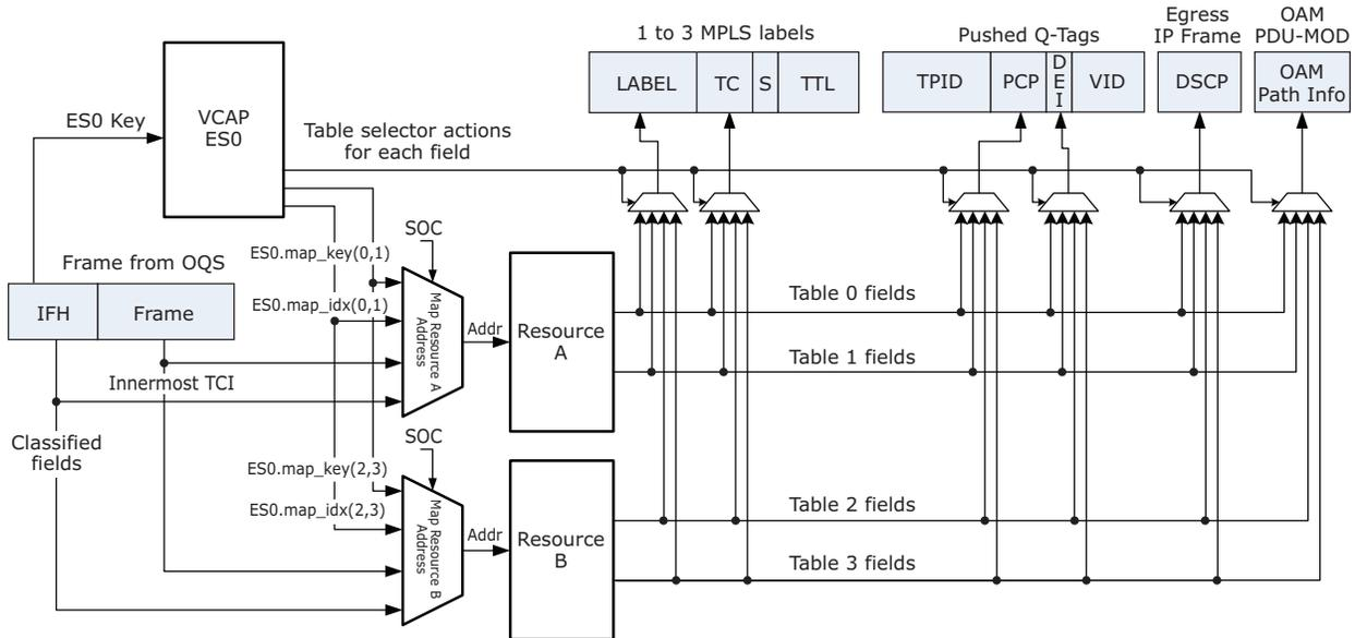
The mapping tables provide a flexible way to update frame fields. The following example shows how to configure and use mapping table 1.
