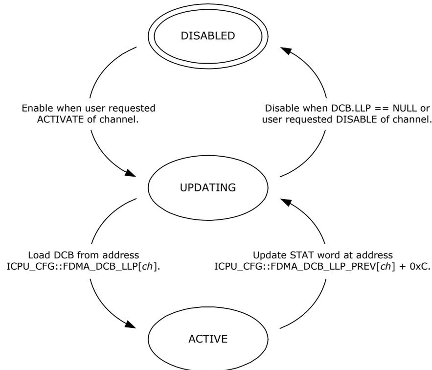
A channel that has `FDMA_DCB_LLP[ch].DCB_LLP==NULL` when going from ACTIVE to UPDATING disables itself instead of loading a new DCB. After this it can be re-enabled as previously described. Extraction channels emit an `INTR_LLPEvent` when loading a DCB with `LLP==NULL`. Injection channels emit an `INTR_LLPEvent` when saving status for a DCB that has the `LLP==NULL`.
