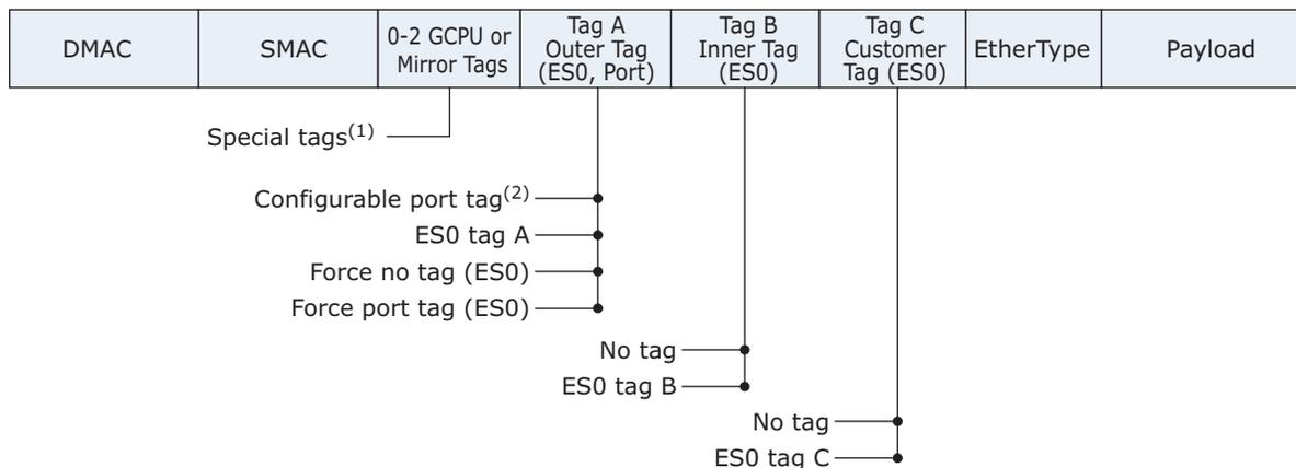
1. Mirror tag is controlled by REW::MIRROR\_PROBE\_CFG.REMOTE\_MIRROR\_CFG.
