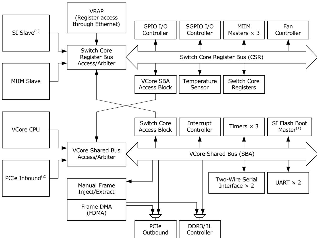
1. When the Vcore-III CPU boots up from the SI Flash, the SI is reserved as boot interface and cannot be used by an external CPU.
