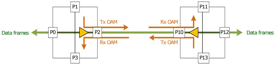
The following illustration shows the detailed frame flow between ports P0 and P2, depicted in the previous illustration. The frame flow from left to right is illustrated at the top of the illustration, and the frame flow from right to left is shown at the bottom.
