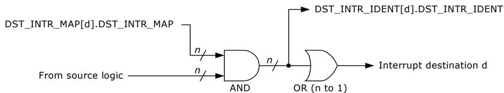
The interrupt destination can enable individual sources for interrupt by writing a mask to `DST_INTR_MAP[ $d$ ].DST_INTR_MAP`. When a source is enabled in `DST_INTR_MAP` then an interrupt from this source will be propagated to the interrupt destination.
