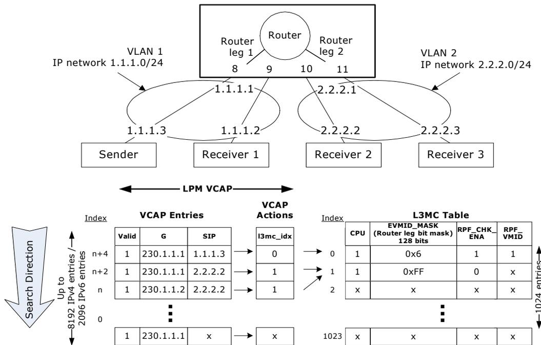
A sender host with IPv4 address 1.1.1.3 is transmitting IPv4 multicast frames to the group address 230.1.1.1 and DMAC = 0x01005E010101. The frames must be L2 forwarded to receivers in VLAN 1 and L3 forwarded to receivers in VLAN 2. For the latter, an entry for the (1.1.1.3, 230.1.1.1) pair is added to the VCAP LPM.
