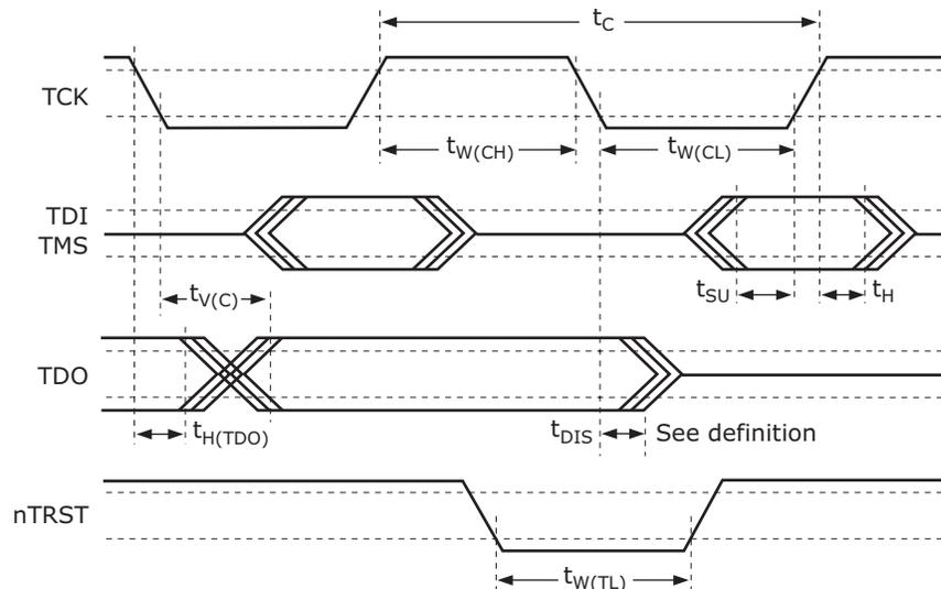
All JTAG signals comply with the specifications in the following table. The JTAG receive signal requirements are requested at the pin of the devices.
