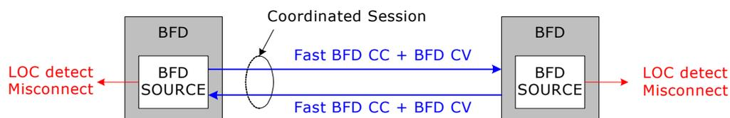
The BFD source checks the incoming BFD CV PDU for misconnectivity in software. If more than a configurable number of BFD CC PDUs are not received, the VOE signals Loss of Continuity (LOC).
