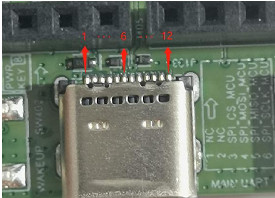
Figure 11: The definition of the Type-C interface (J103)
