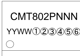
Figure 16. CMT802X Top Marking
