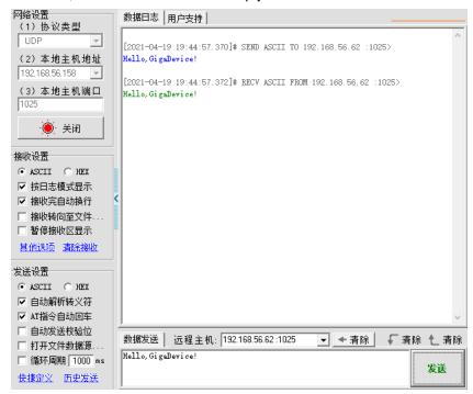
Open the DHCP function in main.h, using a router to connect the board with the pc, users can see the automatic allocated ip address of the board from the HyperTerminal.
