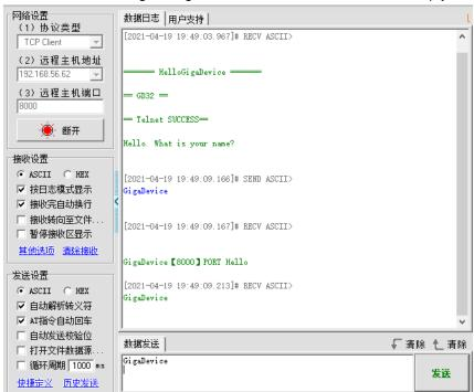
Using Network assistant software, configure the pc side to tcp server, using 10260 port (ensure that the port number is not occupied by other processes), and when send something through the assistant, users can see the echo reply from the client:
