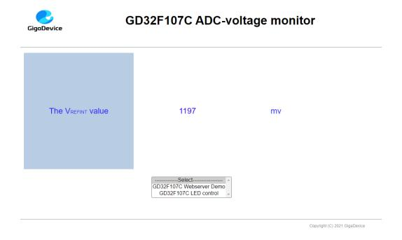
Open the DHCP function in main.h, using a router to connect the board, and use the HyperTerminal to print the automatic allocated ip address, then connect your mobile phone to the wifi which the router send. Users can visit the eval board and control it on your mobile phone.
