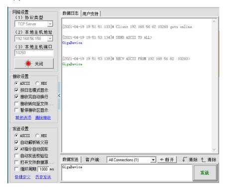
Using Network assistant software, configure to use udp protocol, using 1025 port, and when send something through the assistant, users can see the echo reply from the board:
