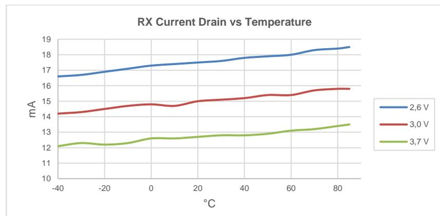
(\*): Consider all graphs as indicative typical results in accordance with temperature variation. Values measured with continuous wave transmission, max power, load 50 Ω.
