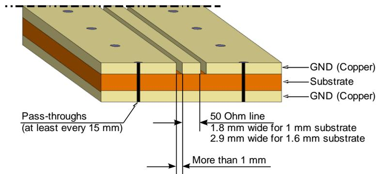
Note: dimensions in the picture above is referred to a FR4 substrate PCB
