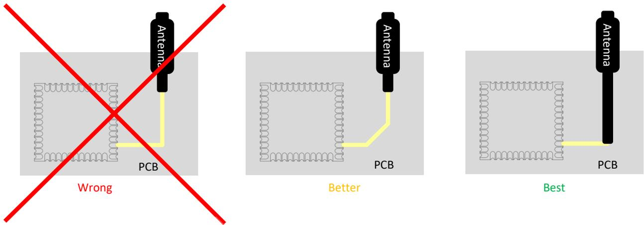
**Figure 11:** Recommended Trace Connects Antenna and the Module
