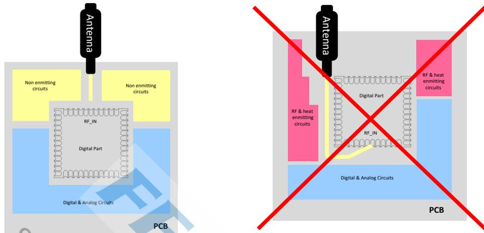
Figure 9: Placement the Module on a System Board
