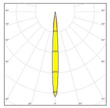
Dimensions: 21.6 mm x 21.6 mm Height: 11.70 mm ~8° spot beam
