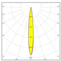
Dimensions: 21.6 mm x 21.6 mm Height: 11.90 mm ~10° diffused spot beam
