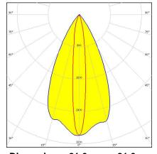
Dimensions: 21.6 mm x 21.6 mm Height: 11.70 mm ~13° x 45° oval beam optimized for Luxeon Rebel. Variant with beam
