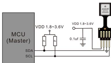
Figure 8. Typical application circuits including pull-up resistance RP and decoupling capacitance between VDD and GND.
