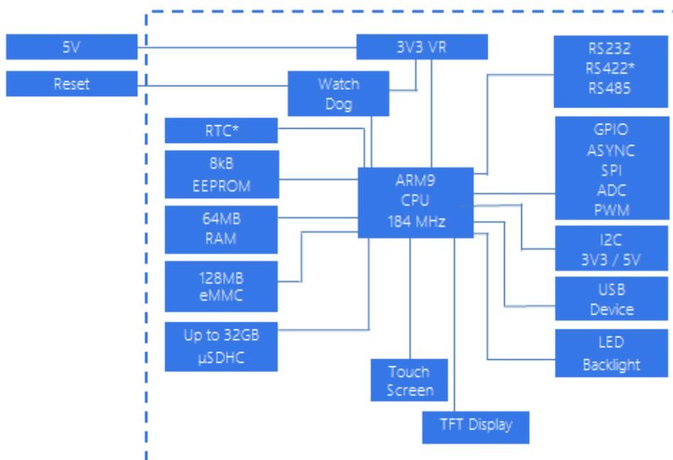
Figure 1 - Circuit Block Diagram.
