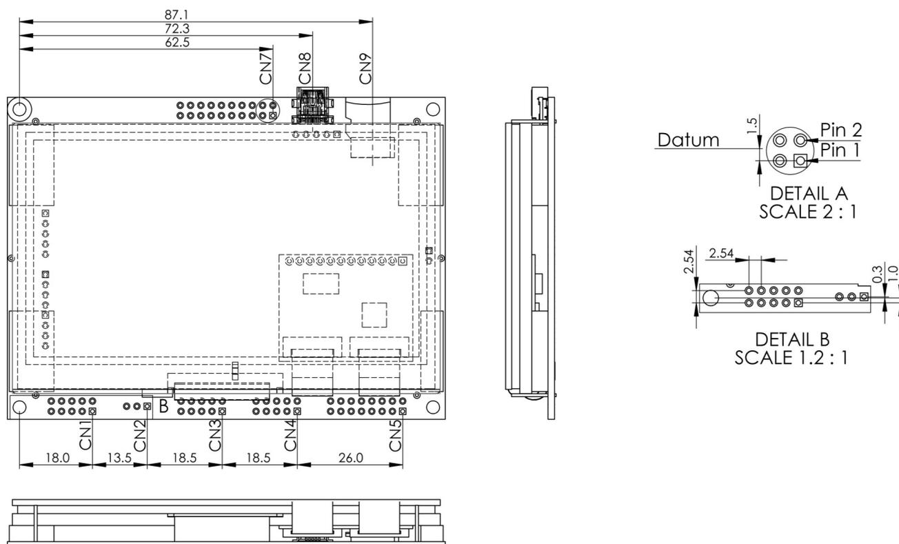
Figure 5 - TU480x272C-K61XA1XX Connector Location drawing. Reference dimensions only.
