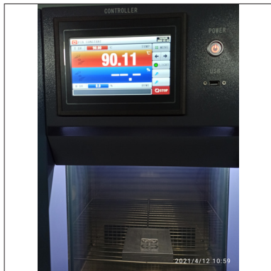
Temperature set in the climatic chamber
