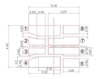
• Tolerance of measurement of the dimension is  $\pm 0.1$ .
