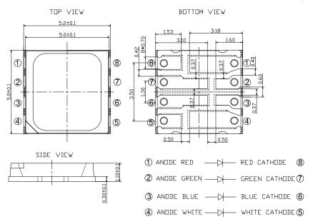
• Tolerance of measurement of the dimension is  $\pm 0.1$ .
