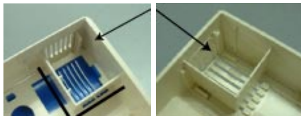
Fig. 19-1 - Example of sensor compartment in detector housing
